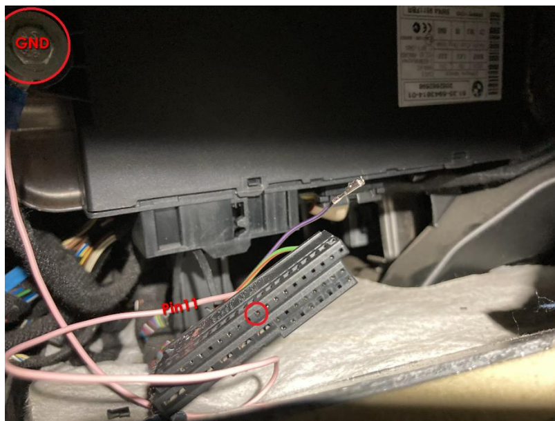
CAS Pin 11 grounding on an E9x manual transmission car
