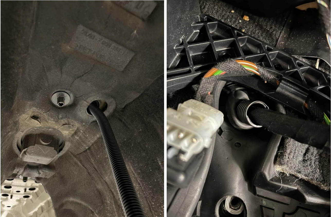
Utilizing the OEM shifter cable passage through the bulkhead
