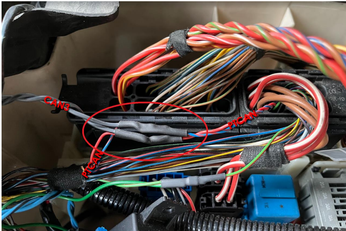
CAN3 wiring spliced into ECU PTCAN (E9x manual transmission car)
