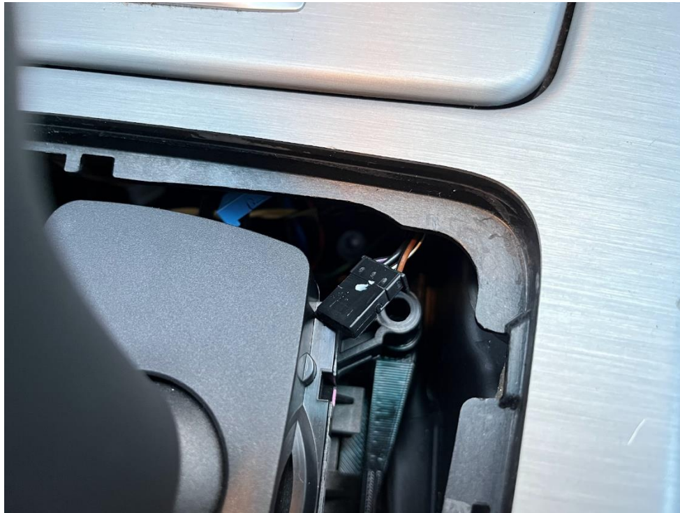
X14275 4-pin connector with PLOCK and ground signals
