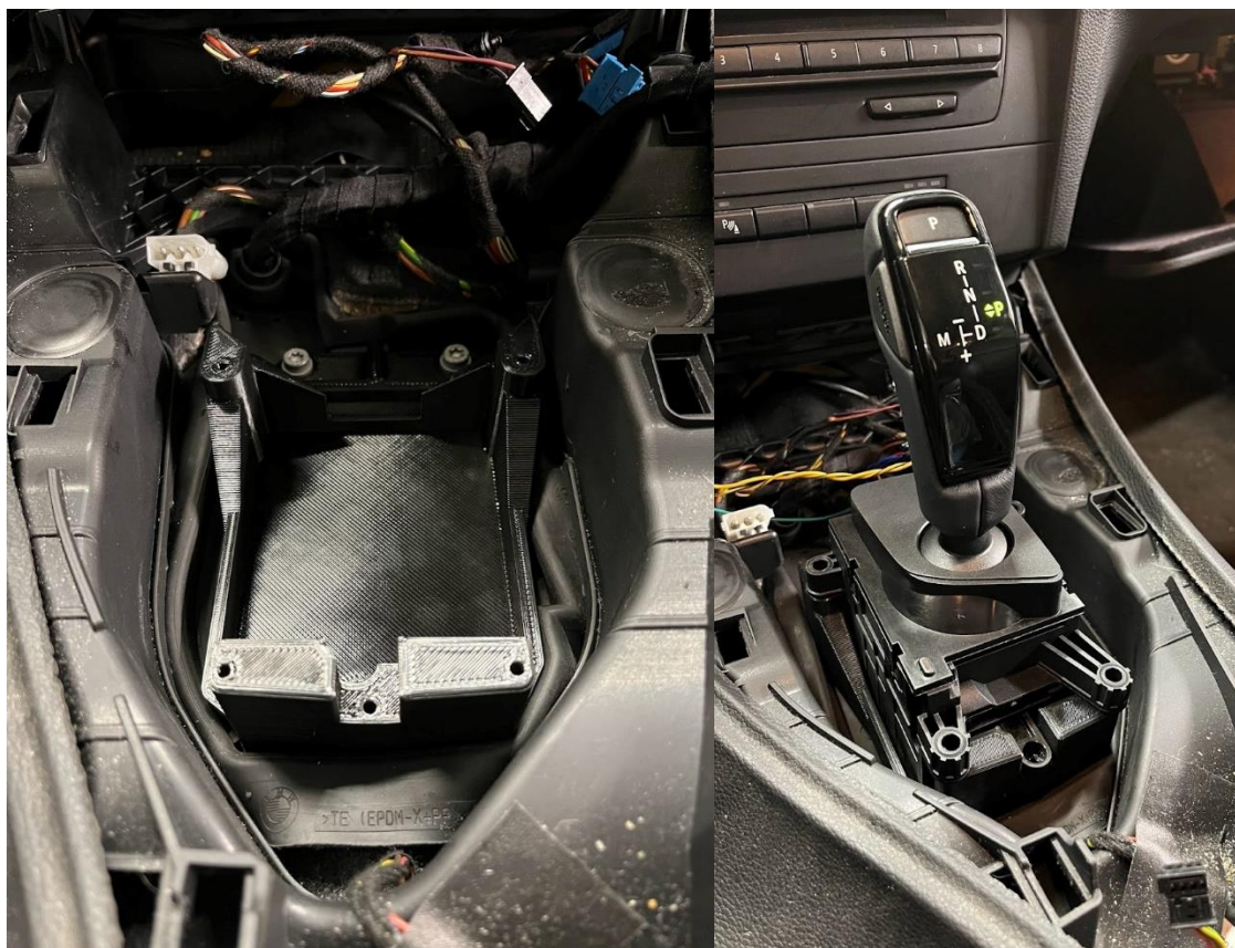
A90 Supra shifter adapter and shifter installed on E9x
