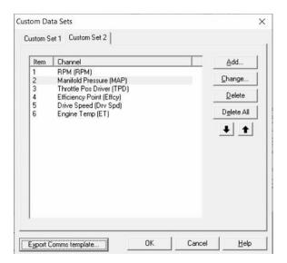
The **Custom Data Set 2** can be broadcasted on either CAN 0 or CAN 1 depending on other devices on the bus. The type of the data set needs to be **Sequential**. Pictured below is the **Custom Data Set 2** configured on CAN 1 as a <u>Custom Data Set 2 Sequential Tx</u>, on <u>Address 1534 (0x5FEh)</u> with a <u>50 Hz Transfer Rate</u>.
