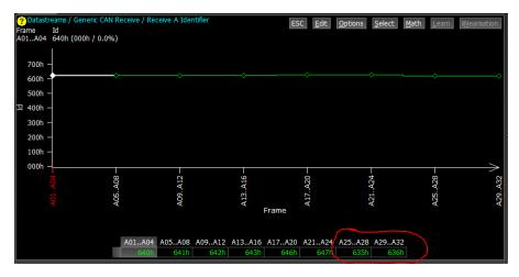
Remember to also enable the frames in Generic CAN Receive -> Receive A Enable and select the correct CAN-bus in Generic CAN Receive -> Receive A Bus.
